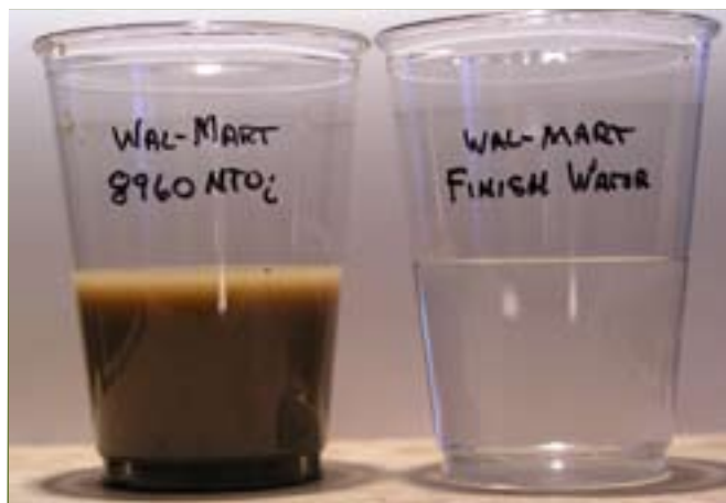
Transformation: site water runoff on left to Floc Log clarification system discharge on right
