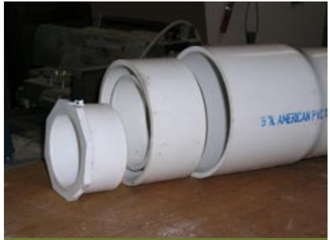
Fig. 5: Housing to down-gradient PVC pipe adaptors
