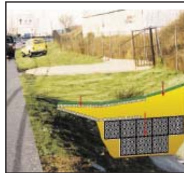
Road Edge Drainage
