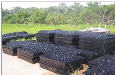
Figure 26: Pre-Assembled GEOTERRA™ Mats
